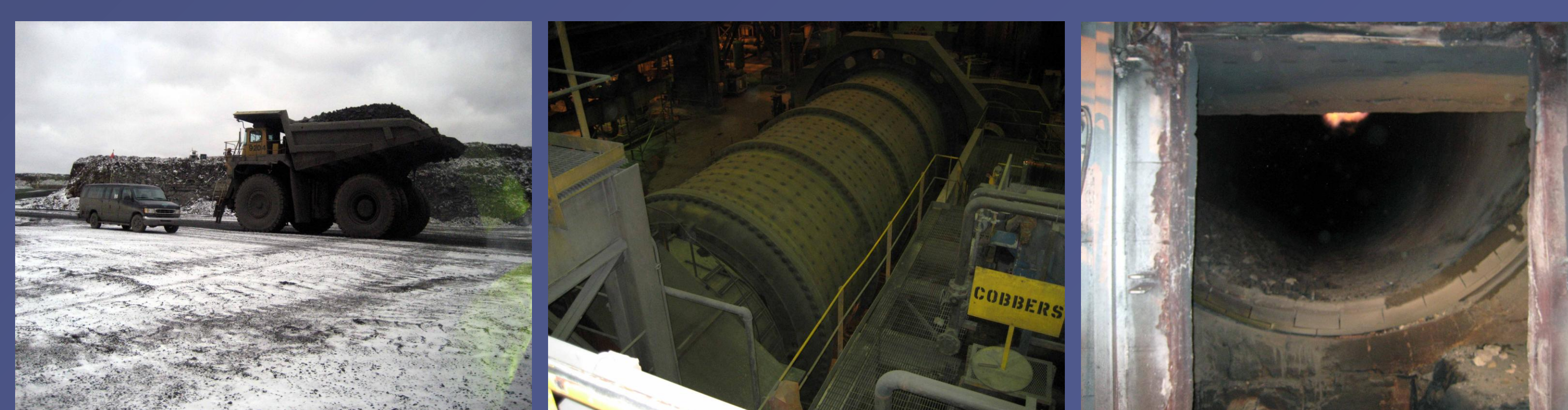
From left: taconite rock collected from open pits, rock is crushed into powder, powder made into pellets and fired
